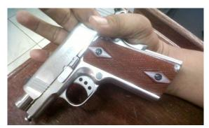
Rack slide back and remove slide stop.
