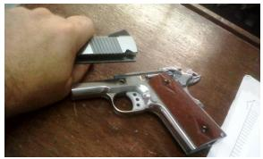
Rack slide forward and remove from frame.
