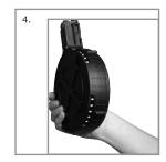
Repeat the procedure until the desired quantity of cartridges is loaded. (max. 110 pcs.)
