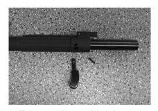
3. Take out the cocking lever first and than the inner tube.
