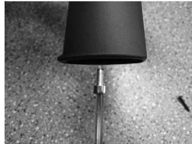
5. Unscrew the inside allen screw in order to remove the trigger group.
